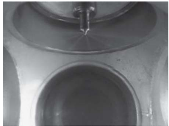
Fig. 5 Image of the fuel-spraying pattern obtained through a CCD camera
